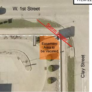
consultation with staff at the lowa DOT, the city has determined the need to retain a 10-foot wide easement over this storm sewer. This easement is essentially 5 feet on both sides of the storm sewer pipe. The remaining portion of the existing easement may be vacated for the new bank facility.
